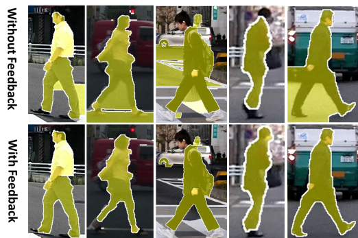
Fig. 12. Result of using feedback. The first row shows the segmentation results without using feedback while the second row shows the results using feedback.
