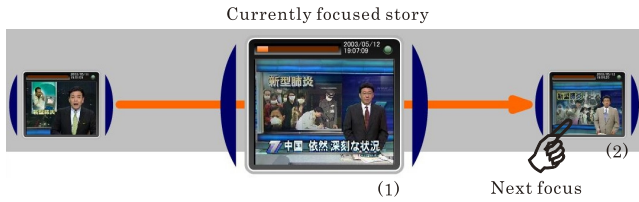
(a) When a thumbnail image that represents a story is clicked, it is enlarged and played. The enlargement is automatically adjusted so that the preceding and the succeeding stories should remain in the screen.
